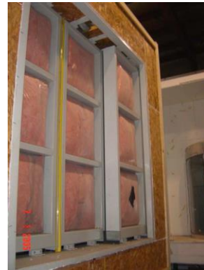
Figure D - Sliding hangar-door mock up in a test chamber
