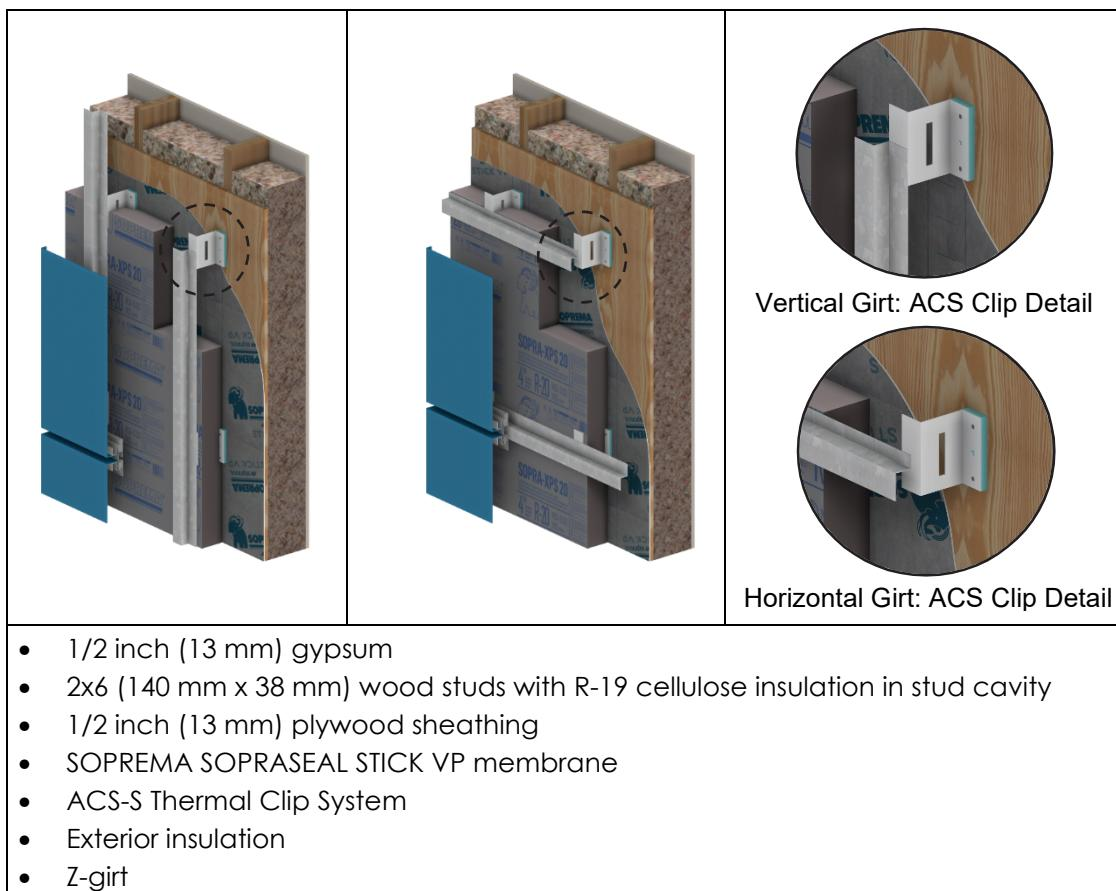
**Figure 1.1:** Schematic of Evaluated ACS-S Thermal Clip with Split Insulated 2x6 Wood Frame Wall Assemblies
